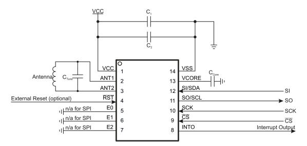
Figure 3. Example Application Diagram (SPI Operation)
