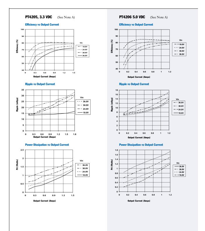
Note A: All data listed in the above graphs, except for derating data, bas been developed from actual products tested at 25°C. This data is considered typical data for the isolated DC-DC converter.
