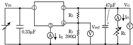
$$V_O = V_{ref} \times \left( 1 + \frac{R_2}{R_1} \right)$$
