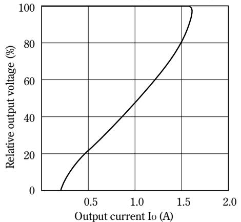
**Fig. 5 Output Voltage Adjustment Characteristics**
