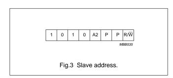
The next significant bit (A2) addresses a particular device. A system could have up to two PCX8598X-2 devices on the bus. The two addresses are defined by the state of the A2 input.
