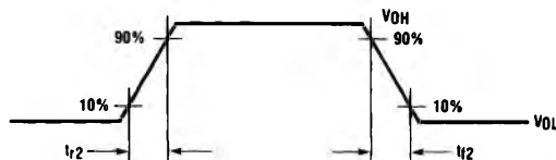
FIGURE 15. Rise and Fall Time Measurement for TA and REG Full
