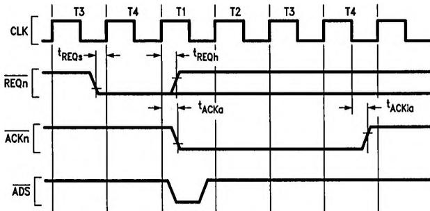
FIGURE 4-16. REQn/ACKn Sequence (DMAC Initially Not Idle)
