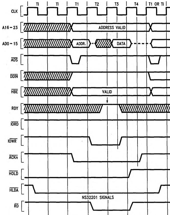
FIGURE 2-6. Direct Memory-To-I/O Data Transfer (Single Transfer Mode)
