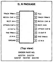
**ELECTRICAL CHARACTERISTICS** Standard Test Conditions (unless otherwise noted)  $V_{CC} = 15V TA = 25^{\circ}C$  Expandor mode (see test circuit) Input signals at unity gain level (OdB) = 100mV RMS at 1KHz,  $V_1 = V_2$ ,  $R_2 = 3.3K$ ,  $R_3 = 17.3K$
