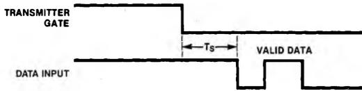
Figure 1. Set-up Time,  $T_S$
