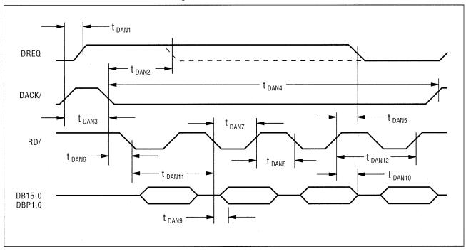
**Burst Mode DMA Read without Byte Control**
