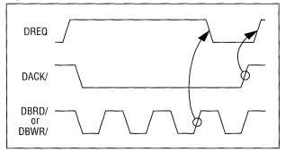
This regular surrendering of the DMA channel has two benefits for two common DMA interface problems. For DMA controllers that do not recognize higher priority requests until the current device finishes, the ASC can
