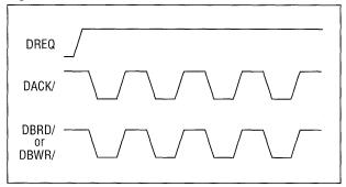
*Normal DMA Mode* illustrates the case where the threshold is always exceeded. This is typical of a DMA interface that is slower than the SCSI device to which the system is connected.
