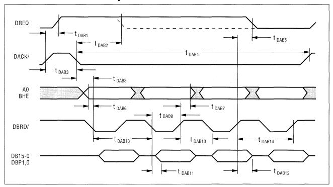
**Burst Mode DMA Read with Byte Control**
