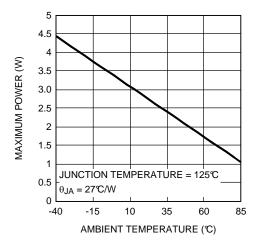
Figure 42. Maximum Dissipation vs. Ambient Temperature
