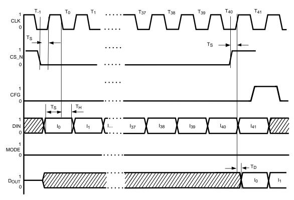
Figure 40. Timing Diagram for Serial Mode
