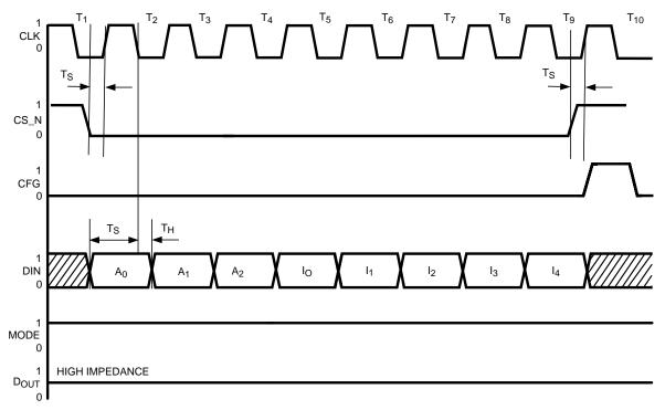
Figure 41. Timing Diagram for Addressed Mode
