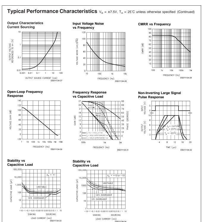
Note: Avoid resistive loads of less than 500  $\!\Omega,$  as they may cause instability.
