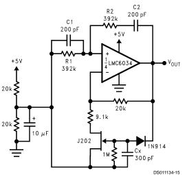
Oscillator frequency is determined by R1, R2, C1, and C2: fosc =  $1/2\pi$ RC, where R = R1 = R2 and
