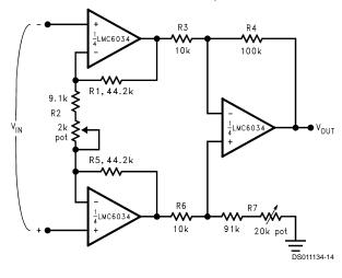
$$\frac{V_{OUT}}{V_{IN}} = \frac{R2 + 2R1}{R2} \times \frac{R4}{R3}$$
