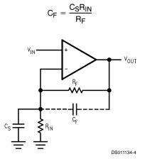
$C_S$  consists of the amplifier's input capacitance plus any stray capacitance from the circuit board and socket.  $C_F$  compensates for the pole caused by  $C_S$  and the feedback resistors.
