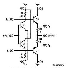
Pin numbers in parentheses denote pin connections for dual-in-line package.
