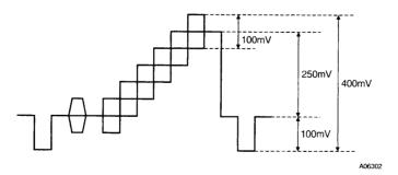
14. Apply a 5-step staircase wave (as in the figure below) to Y-IN, and measure the luminance level (Y) and the sync level (S) in the Y-OUT output.
