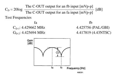
5. Measure the C-OUT output when a 200-mVp-p sine wave is input to C-IN1 and C-IN2, and when a 500-mVp-p sine wave is input, and calculate the gain difference as follows:
