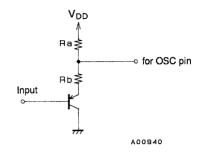
Use the LB1871  $V_{REG}$  output for the  $V_{DD} = 6.3 \text{ V}$  case.
