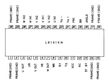
Note: All FRAME pins are connected to GND.
