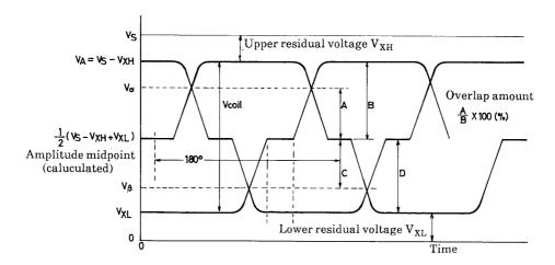
$$\begin{array}{l} Upper\ overlap = & (2V\alpha - V_A - V_{XL}) \,/\, (V_A - V_{XL}) \times 100[\%] \\ Lower\ overlap = & (V_A + V_{XL} - 2V\beta) \,/\, (V_A - V_{XL}) \times 100[\%] \end{array}$$
