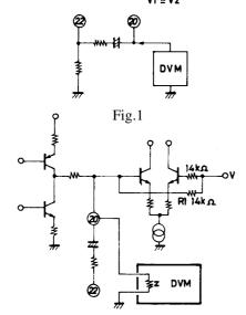
Note : When adjusting by this method, use a DVM (digital voltmeter) with high input impedance. At Zi=10M $\Omega$ , the adjustment error is approximately 20kHz, The error ( $\Delta V$ ) with the DVM connected is.
