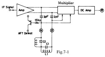
C2 forms a sound trap for preventing malfunction of the AFT.
