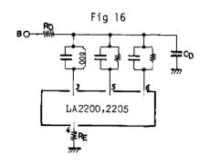
Each signal's attenuation in dB is given as mentioned above. To prevent actual interference, it must be considered that levels of AF signal and BK, DK signal differ extremely. Too much interference causes undesirable phenomena to occur as shown below.
