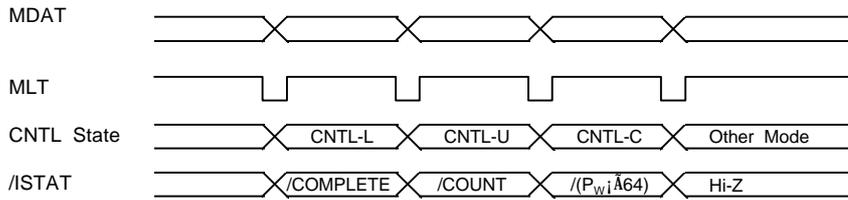
Fig 7.  $\overline{ISTAT}$  output signal according to CNTRL Register
