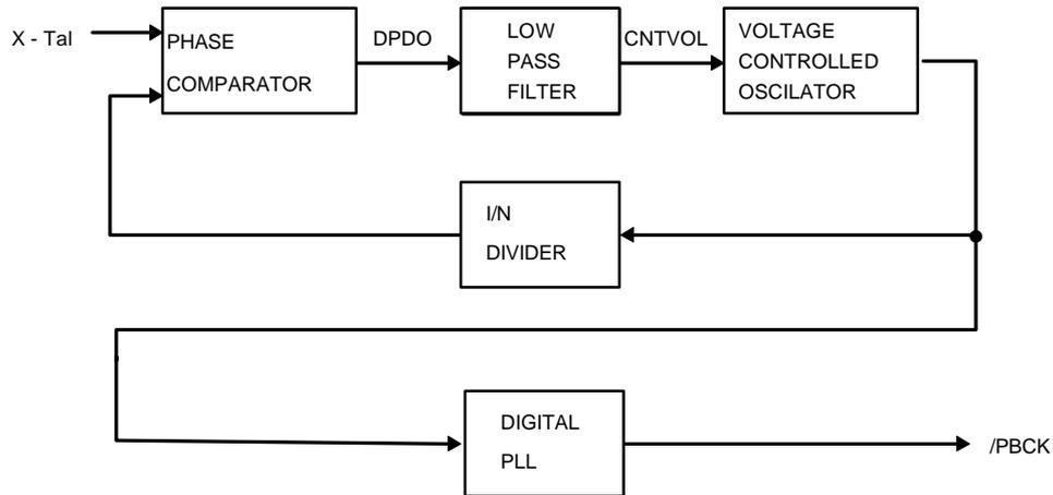
Fig. 21: The application diagram of Digital PLL
