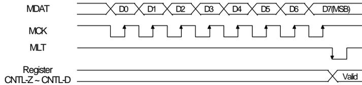
Fig. 5 : Micom data input timing chart
