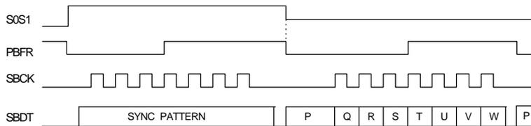
Fig 16. Timing chart of digital audio out
