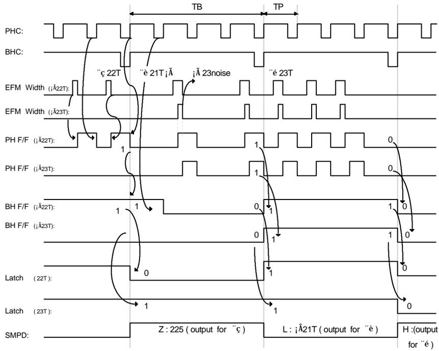
FIG.20 : Timing chart of SMPD output when the gain is "H" in the speed mode
