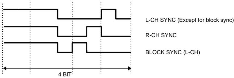
Fig 15. Preamble signal
