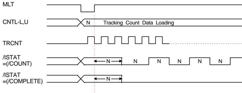
Fig. 6 : Tracking Counter Timing Chart
