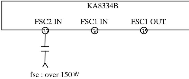
\* Serial data selection : FSC2 → ON, FSC1 → OFF (cf. S-DATA table)
