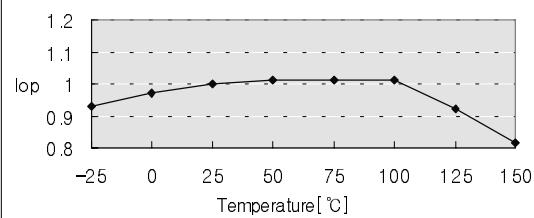
Fig.4 Max Inductor Current
