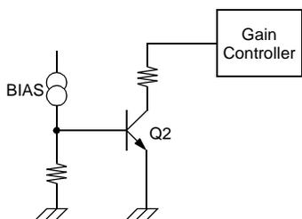
When the chip temperature rises up to about 175°C, the Q2 turns on so that the output driver will be shutdown. When the chip temperature falls off to about 150°C, then the Q2 turns off so that the driver is to operate normally. Thus, TSD has the temperature hysteresis of about 25°C.
