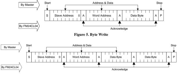
Figure 6. Multiple Byte Write
