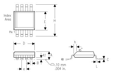
Controlling dimensions in millimeters. Conversions to inches are not exact.
