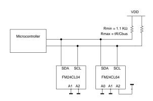
Figure 2. Typical System Configuration
