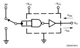
$I_{\mbox{OS}}$  is tested for both input conditions at each of the specified output conditions.
