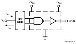
When testing  $I_{\text{IH}},$  the other input is at 3V; when testing  $I_{\text{IL}},$  the other input is open.
