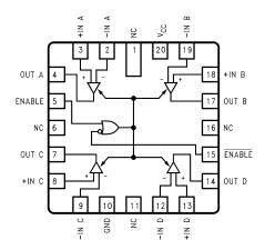
Figure 2. 20-Lead Ceramic Leadless Chip Carrier
