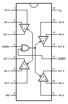
Figure 1. 16-Lead DIP Top View
