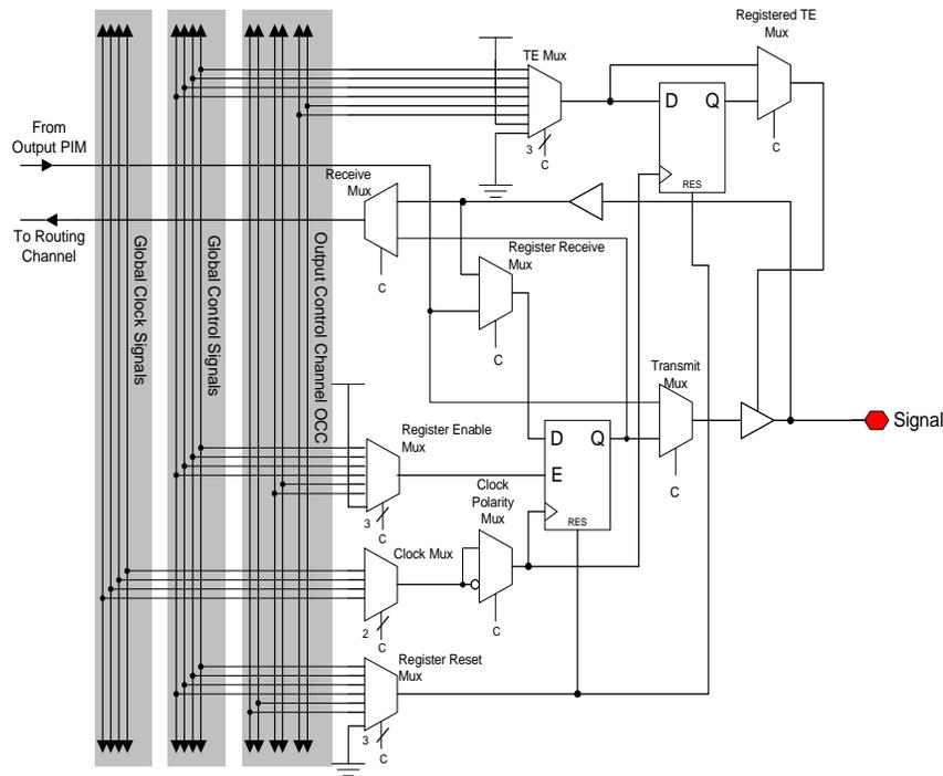
**Figure 2. Block Diagram of a Standard Datapath Cell**
