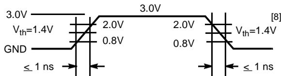
(c) LVTTL Input Test Waveform
