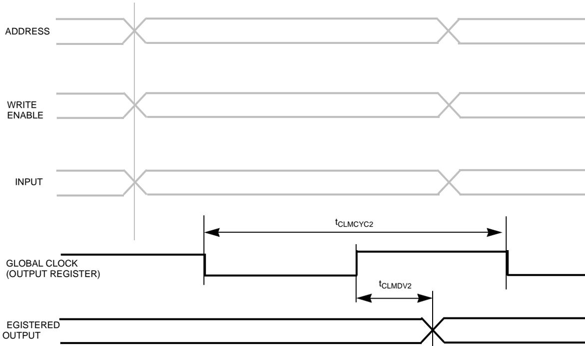
**Cluster Memory Output Register Timing (Synchronous Inputs)**
