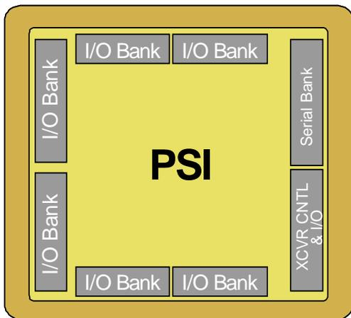
**Figure 8. PSI I/O Bank Block Diagram**
