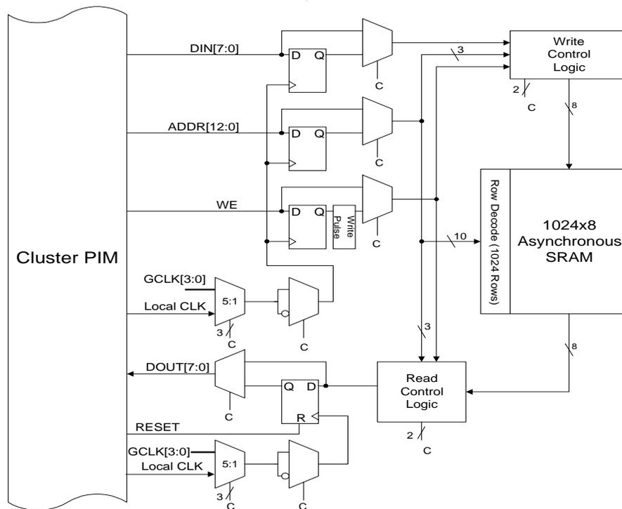
**Figure 6. Block Diagram of Cluster Memory Block**
