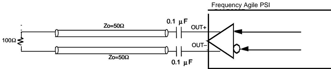
**Figure 17. Serial Output Termination**
