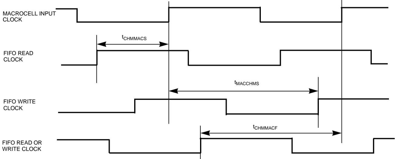
**Channel Memory DP SRAM Flow Through R/W Timing**
