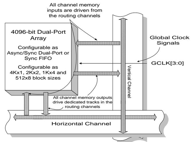
**Figure 7. Block Diagram of Channel Memory Block**
