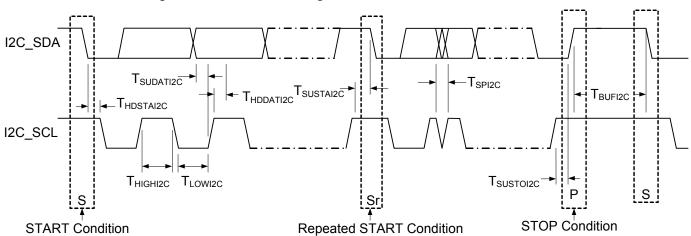
Figure 10. Definition of Timing for Fast/Standard Mode on the I<sup>2</sup>C Bus
