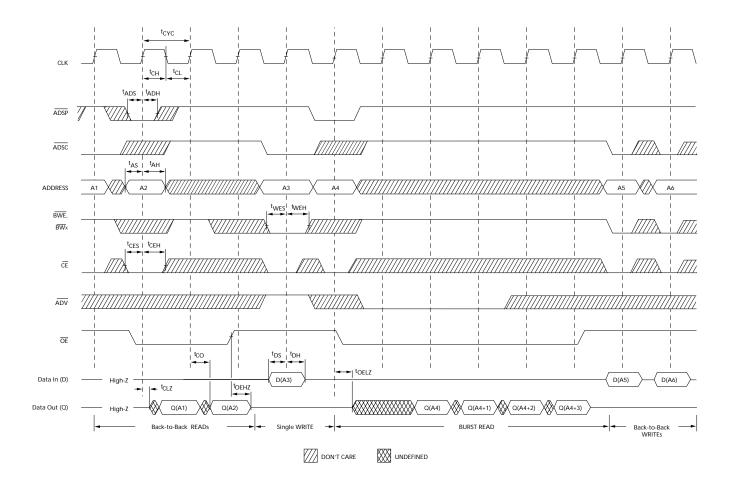
29. On this diagram, when  $\overline{CE}$  is LOW:  $\overline{CE}_1$  is LOW,  $\overline{CE}_2$  is HIGH and  $\overline{CE}_3$  is LOW. When  $\overline{CE}$  is HIGH:  $\overline{CE}_1$  is HIGH or  $\overline{CE}_2$  is LOW or  $\overline{CE}_3$  is HIGH. 30. The data bus (Q) remains in high Z following a WRITE cycle, unless a new read access is initiated by ADSP or ADSC. 31. GW is HIGH.
