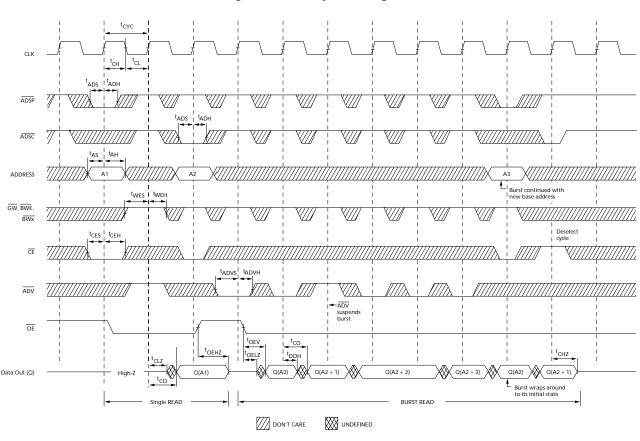
26. On this diagram, when  $\overline{CE}$  is LOW:  $\overline{CE}_1$  is LOW,  $\overline{CE}_2$  is HIGH and  $\overline{CE}_3$  is LOW. When  $\overline{CE}$  is HIGH:  $\overline{CE}_1$  is HIGH or  $\overline{CE}_2$  is LOW or  $\overline{CE}_3$  is HIGH.
