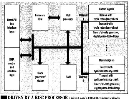
DRIVEN BY A RISC PROCESSOR, Cirrus Logic's CD2400 communications peripheral chip has four full-multiplexed channels, each of which can handle a different protocol. Modem control logic and bit-rate generators within each channel allow users to select the protocol and transmission rate desired.
