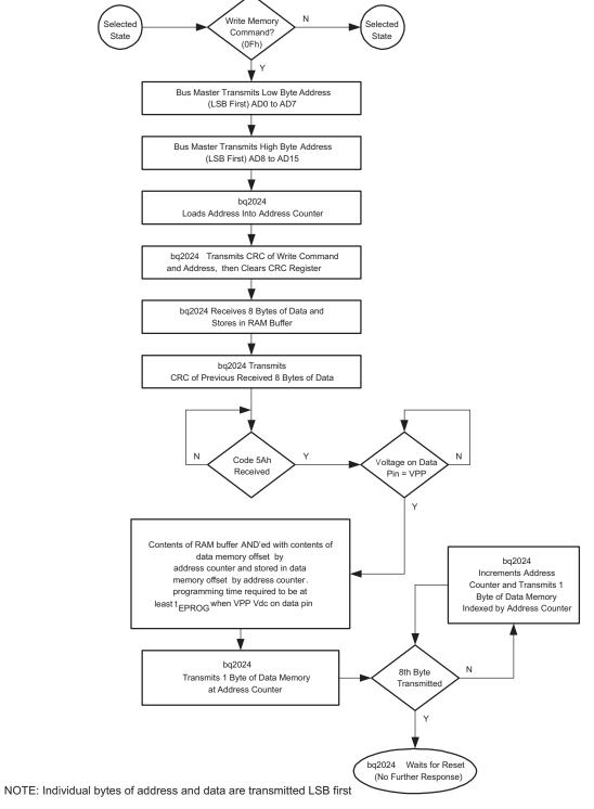
Figure 9. WRITE MEMORY Command Flow
