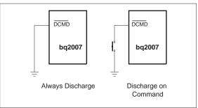
Figure 3. Discharge-Before-Charge
