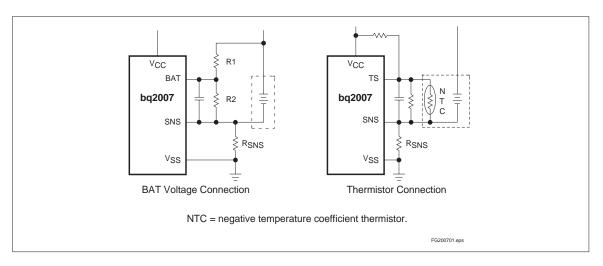
Figure 2. Voltage and Temperature Limit Measurement
