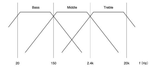
The input signal is separated into three regions : bass (20Hz to 150Hz), middle (150Hz to 2.4kHz) and treble (2.4kHz to 20kHz). These regions are then joined again with the middle and treble regions phase shifted -180° and -360° respectively with respect to the bass signal. This phase shift adjusts the delay time characteristic for each band and minimizes the distortion of the rising section of the audio signal.
