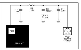
Figure 5. Loop Filter Circuit Diagram
