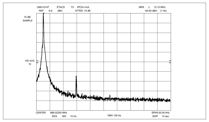
Figure 9. Typical Carrier Spectrum – 50kHz Span
