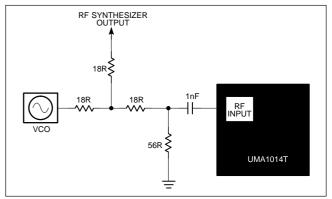
Figure 4. RF Power Splitter Circuit Diagram
