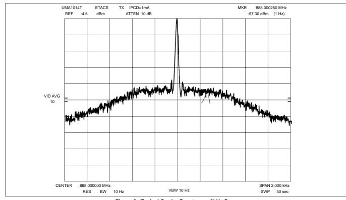
Figure 8. Typical Carrier Spectrum – 2kHz Span
