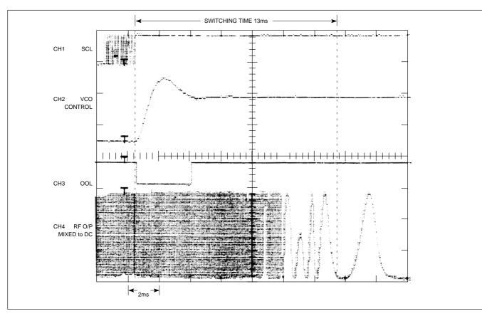
Figure 10. Typical Switching Waveforms
