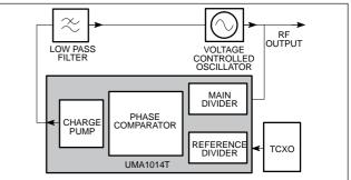
Figure 1. PLL Circuit Block Diagram
