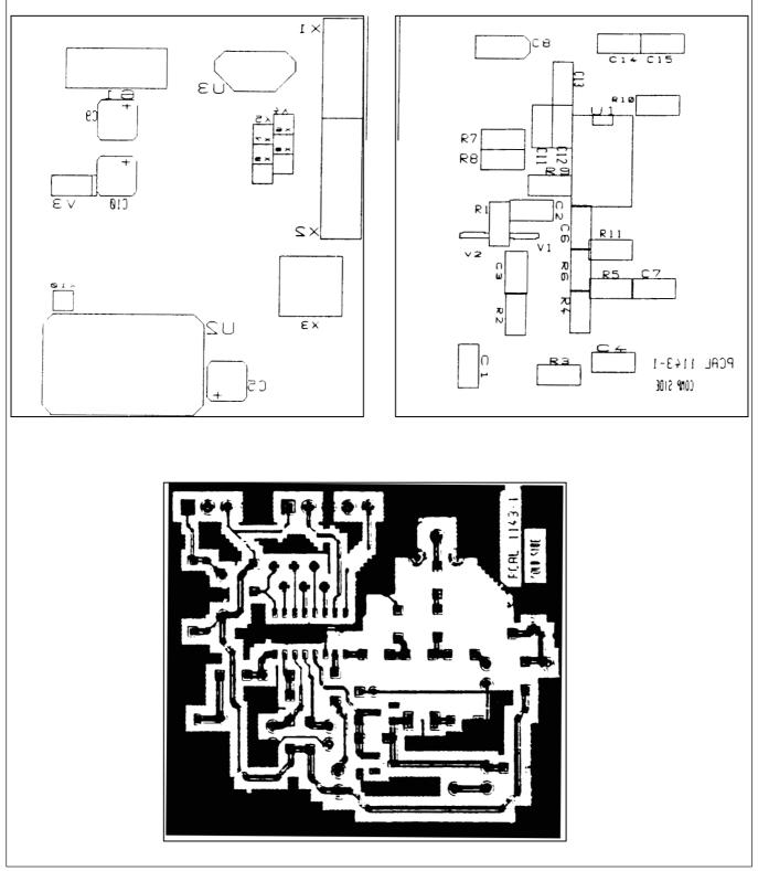
Figure 7. Board Layout for UMA1014T Frequency Synthesizer
