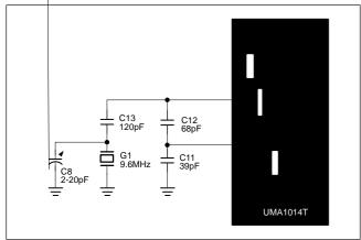
Figure 3. Crystal Oscillator Circuit Diagram
