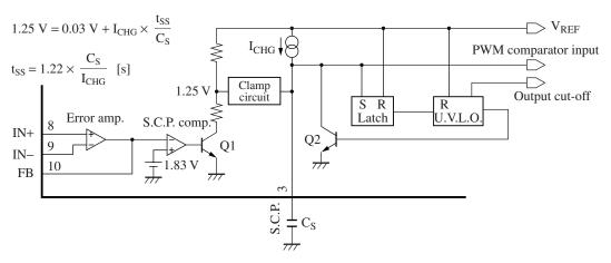
Figure 6. Short-circuit protection circuit
