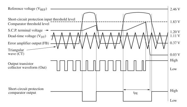
Figure 2. Short-circuit protection operation waveform
