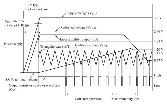
Figure 1. PWM comparator operation waveform
