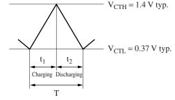
Figure 4. Triangular wave oscillation waveform
