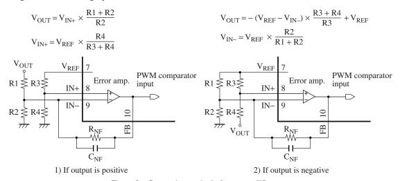
Figure 3. Connection method of error amplifier
