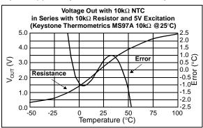
**FIGURE 6:** The series configuration response of the circuit shown in Figure 5a. has good linear response in a  $\pm 25^{\circ}$ C range surrounding the temperature where both resistors (NTC and  $R_{SER}$ ) are equal. The error in this range is typically within  $\pm 1\%$ . VREF = 5V.
