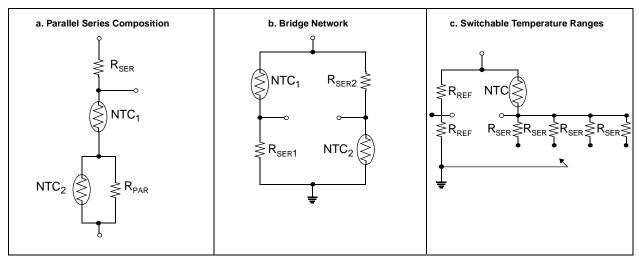
FIGURE 9: Other Thermistor Linearization Circuits.
