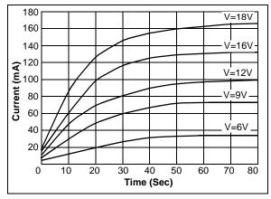
**FIGURE 2:** The time constant of the thermal mass of the thermistor sensor can be used to time delay a reaction to changes in conditions in a circuit. If a thermistor is overdriven, the thermal mass time constant of the sensor eventually causes the thermistor to overheat, reducing its resistance.
