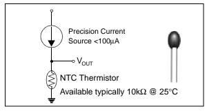
**FIGURE 4:** Common sense would dictate that the thermistor be excited by a precision constant current source as shown in this figure. A picture of an NTC Thermistor is shown on the right.
