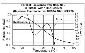
**FIGURE 7:** The parallel configuration response of the circuit shown in Figure 5c. allows for a counter to be used to determine the relative resistance of the NTC element.
