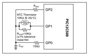
**FIGURE 12:** This circuit switches the voltage reference on and off at GP1 and GP2. In this manner, the time constant of the NTC Thermistor ( $R_{NTC} \parallel R_{PAR}$ ) and integrating capacitor ( $C_{INT}$ ) is compared to the time constant of the reference resistor ( $R_{REF}$ ) and integrating capacitor.
