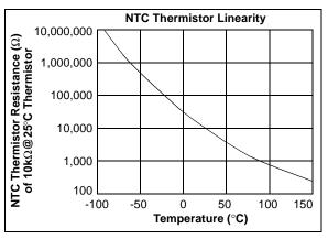
**FIGURE 3:** In precision temperature measurement environments, the thermistor is used in a "zero power" condition. In this condition, the power consumption of the thermistor has a negligible affect on the elements resistance. This is a graph of an NTC  $10k\Omega$  thermistor resistance-versus-temperature.
