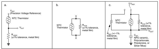
**FIGURE 5:** The series configuration (a) requires a voltage excitation. The parallel configuration (b) can be used in the feedback loop of an amplifier and does not require a precision source. The parallel configuration can be combined with a capacitor (c) which provides a linear circuit response with time.
