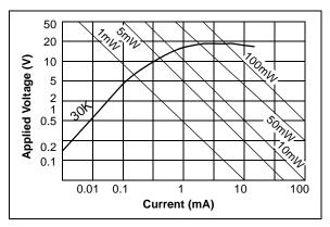
**FIGURE 1:** When a thermistor is overheated by its own power, the device operates in the voltage-versuscurrent mode. In this mode, the thermistor is best suited to sense changes in the ambient conditions, such as changes in the velocity of air flow across the sensor.
