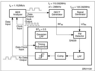
Figure 9. Block Diagram of the BER Evaluation Set-up
