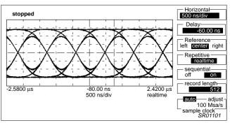
Figure 10. Recovered Eye-Diagram at the Output of SA639
