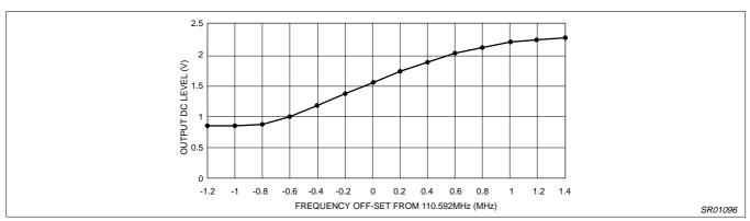
Figure 5. Quad Tank S-Curve of SA639 Board
