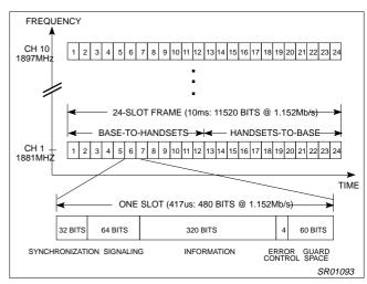
Figure 1. DECT TDD/TDMA Frame Structure
