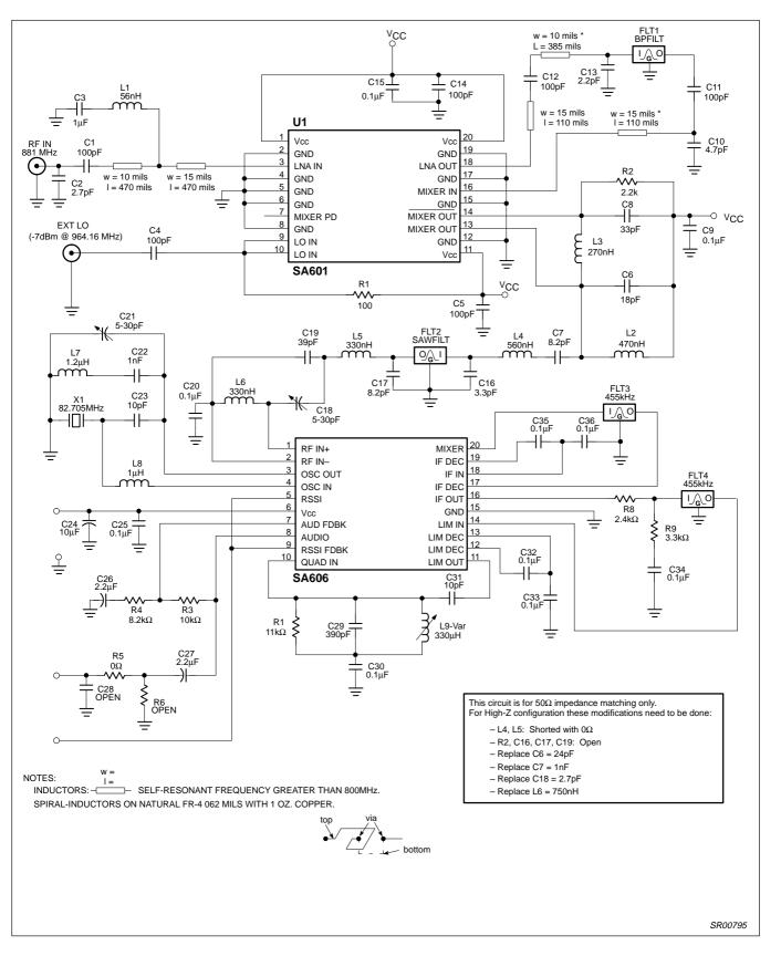
Figure 3. Schematic of the SA601/SA606 Demoboard
