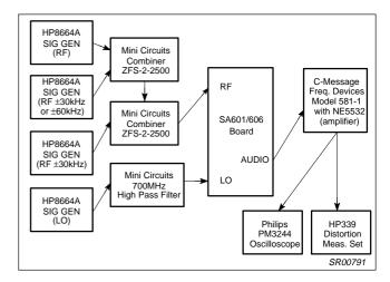
Figure 10. Test Setup for Measuring RF Sensitivity, Adjacent and Alternate Channel Rejection and Spurious Rejection
