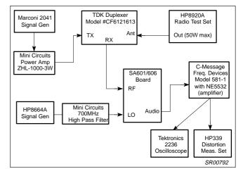
Figure 11. Test Setup for Measuring Transmitter
