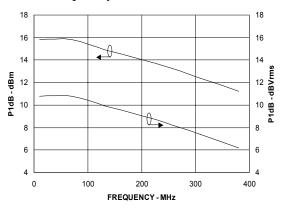
TPC 5. Output Compression Point versus Frequency at Maximum Gain
