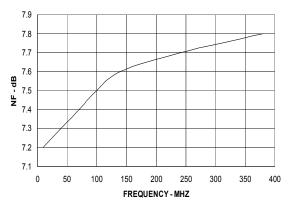
TPC 6. Noise Figure versus Frequency at Maximum Gain
