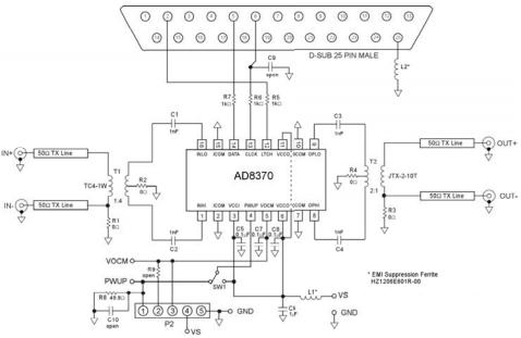
Figure 5. AD8370 Evaluation Board Schematic
