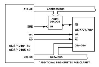
Figure 9. AD7776/AD77778 to ADSP-2101 and ADSP-2105 Interface
