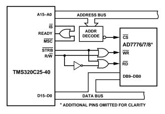
Figure 8. AD7776/AD7777/AD7778 to TMS320C25 Interface
