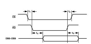
Figure 1. Read Cycle Timing
