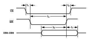
Figure 2. Write Cycle Timing
