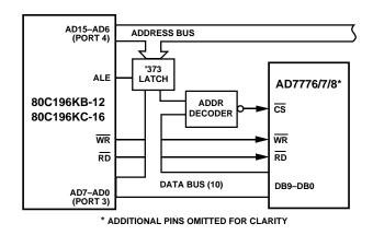
Figure 10. AD7776/AD7777AD7778 to 80C196 Interface
