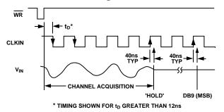
Figure 6. ADC Conversion Start Timing
