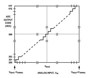
Figure 5. ADC Transfer Function
