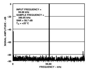
Figure 11. ADC FFT Plot
