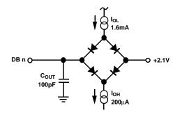
Figure 4. Load Circuit for Bus Timing Characteristics
