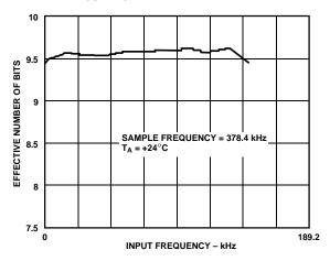
Figure 12. Effective Number of Bits vs. Frequency
