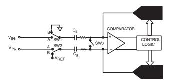
Figure 5. ADC Conversion Phase
