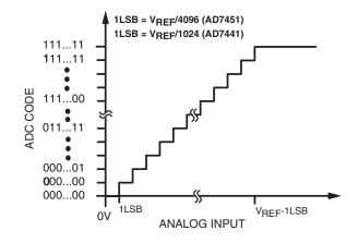
Figure 6. AD7451/AD7441 Ideal Transfer Characteristic
