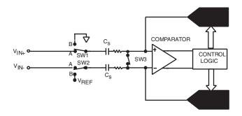
Figure 4. ADC Acquisition Phase
