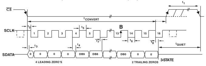
Figure 2. AD7441 Serial Interface Timing Diagram
