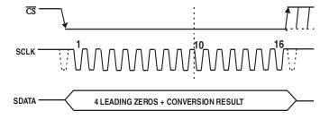
Figure 13. Normal Mode Operation
