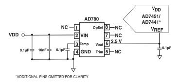
Figure 11. Typical  $V_{REF}$  Connection Diagram for  $V_{DD} = 5 V$
