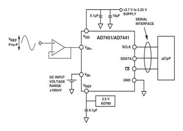
Figure 7. Typical Connection Diagram
