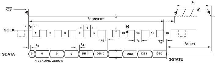
Figure 1. AD7451 Serial Interface Timing Diagram
