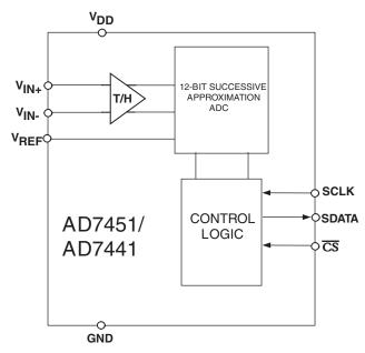
The AD7451/AD7441 use advanced design techniques to achieve very low power dissipation at high throughput rates.
