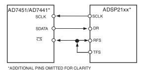
Figure 16. Interfacing to the ADSP 21xx
