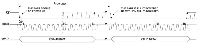
Figure 14. Exiting Power Down Mode
