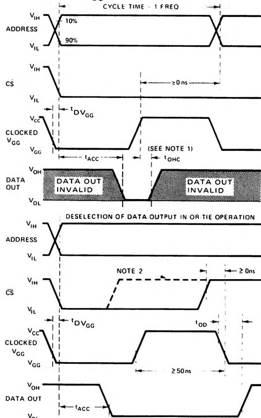
NOTE 1: The output will remain valid for  $t_{OHC}$  as long as clocked  $V_{GG}$  is at  $V_{CC}$ . An address change may occur as soon as the output is sensed (clocked  $V_{GG}$  may still be at  $V_{CC}$ ). Data becomes invalid for the old address when clocked  $V_{GG}$  is returned to  $V_{GG}$ .
