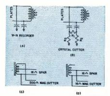
Fig. 7. Change in output wiring for feeding different types of recorders.
