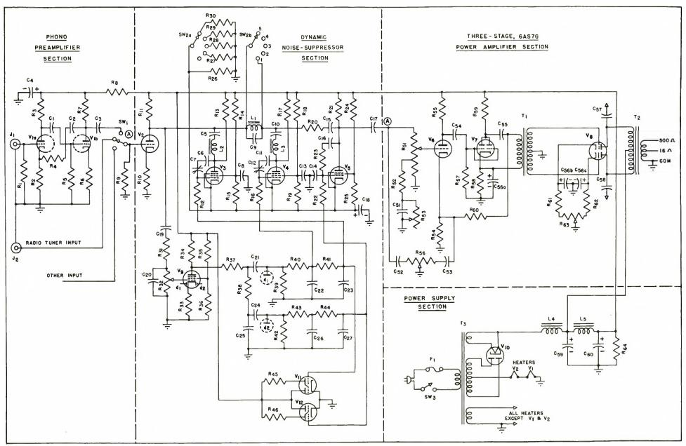
Fig. 5. Complete schematic for the sectionalized amplifier. By combining desired sections, practically any requirements may be met.  $V_1$ —12SL7GT,  $V_2$ —12J5GT,  $V_3$ ,  $V_4$ ,  $V_4$ —6AB7,  $V_5$ —6AB7,  $V_5$ —6AB7,  $V_7$ —6E5.
