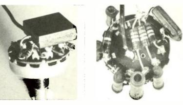
Fig. 4. Assembly of tone controls on standard switches to provide units easily wired into the control section. Left—bass control; right—treble control.
