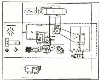
Fig. 6. Partial wiring diagram of power section to show component mounting.
