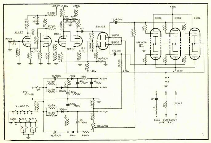
Fig. 1. This is the complete schematic diagram of the transformerless amplifier. Its total cost is comparable to that of a single high-quality out put transformer. For safety, use of a 1-to-1 isolation transformer is recommended between the a.c. line and the power input terminals.
