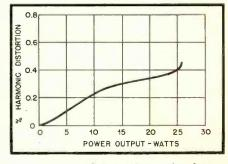
Fig. 3. Harmonic distortion is less than 0.4 per cent at the related output of 20 watts into a 16-ohm speaker. Intermodulation measurements would mean little since there are no frequencysensitive nonlinear elements in the design.
